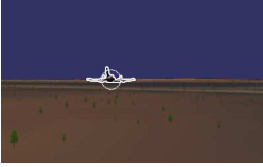
Fig. 3. Sample segmentation using active contour. The initial contour is the white dotted circle and the final contour is the white line surrounding the airplane.
