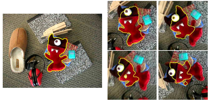
Fig. 10. Unsuccessful tracking using a static base mask. If the base mask is formed from initial upright segmentation ( left ), the basin of attraction is too narrow and so tracking fails to fully capture the object as it rotates. Full image ( left ) and selected cropped frames showing failure to capture the full object ( right ).
