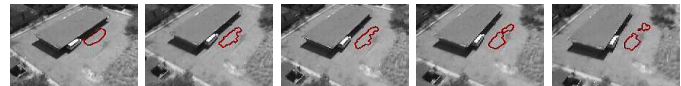
Fig. 15. Selected consecutive frames from the aerial van sequence demonstrating the failure of the level set method to track under a large displacement. Since this technique is more local, once one frame is significantly off, it is unable to search far enough to recover the van and so remains off.
