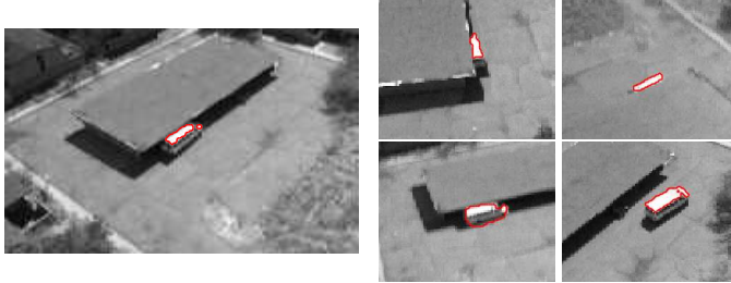
Fig. 13. Tracking a van from a helicopter-mounted camera circling overhead. Full image (left) and selected cropped frames (right).
