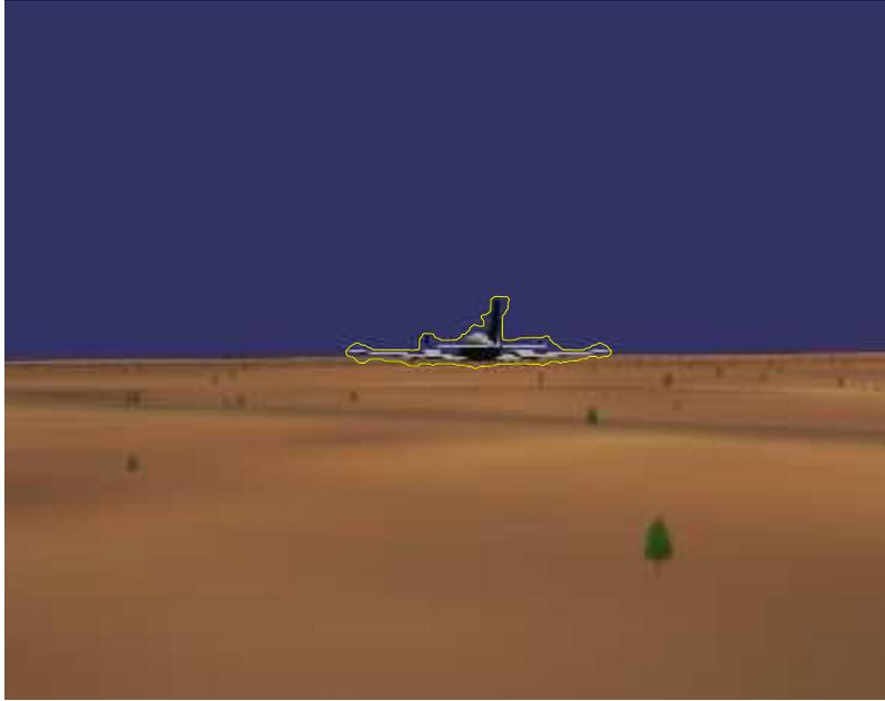
Figure 5. A frame of a simulated leader-follower scenario, as seen from the follower camera. The yellow contour is estimated by the visual observer.
