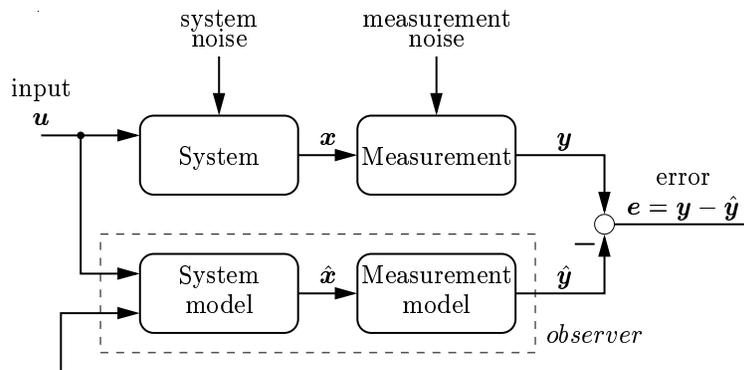
**Figure 3. General Observer Structure.** The error  $e$  is implicitly defined by means of the correspondence procedure. The measurement makes use of standard segmentation algorithms and the prediction part is given by a chosen prior.
