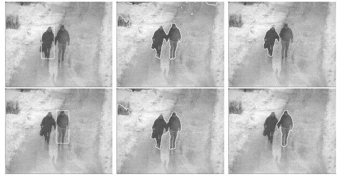
Fig. 6. Couple of similar intensity showing leaking in absence of shape prior: initial, without shape, with shape.
