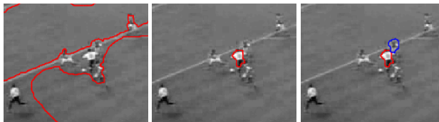
Figure 1: Tracking two interacting soccer players among others of similar intensity: no distance penalty and applying distance penalty to track one or two players (left to right). Without the distance penalty, multiple non-intended regions were captured.
