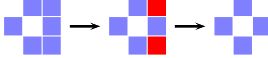
Figure 6. During cleanup, unnecessary interface points (red) are detected and removed to ensure minimal interface.
